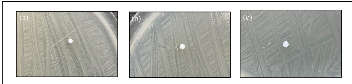
Figure 3. Results of S. aureus inhibition in each sample: (a) Control PLA (b) PLA-PDA and (c) PLA-PDA-everolimus
